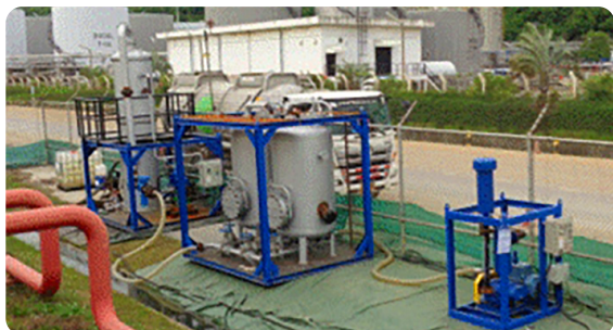
Scrubber Unit Machine, developed to reduce VOCs emissions during oil storage tank maintenance in 2023
